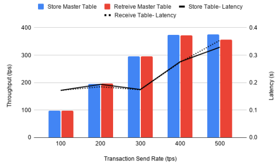
Figure 3: Transaction throughput and latency for the main blockchain layer
